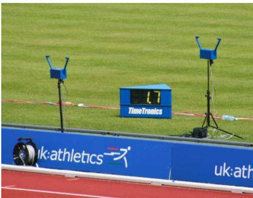
WindSpeed is the first commercial wind-gauge for athletics which specifically applies the principle of electronic and sonic wind speed measurement.
